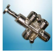
The Model 200 and 201 air interlock valves are installed on bottom loading adaptors and vapor recovery fittings to lock the brakes to prevent driveaways during loading. Pneumatic valves can be used in a number of different applications for additional safety features.
