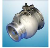
Civacon's 633LVB high-flow, low pressure drop poppeted vapor recovery fitting permits simultaneous multiple compartment loading at +1000GPM without exceeding the pressure rating of the PV vents. The same high-flow design delivers faster unloading, too.
