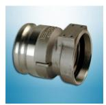
Our 611 Series poppeted vapor recovery or 610 Series non-poppeted vapor recovery adaptors contain the vapors and condensation within the vapor line, minimizing unwanted driver exposure and vapor loss into the atmosphere. The poppet design also ensures that vapor lines are properly connected during unloading.
