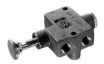
Play it safe with this lightweight valve that locks up the brakes on the trailer, preventing it from leaving the loading rack while connected to the loading arm. This three-way air valve can be used normally open or normally closed, has an adjustable stem, and comes with standardized TTMA and API mounting holes. The anodized aluminum valve is used on all API bottom loading adapters and all Vapor Check Valves.
