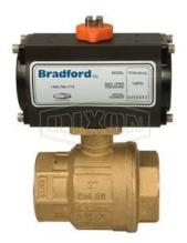
Available in ¼"-4" NPT threaded. Available in brass and stainless bodies. They are available in 2 way and 3 way configurations. Air to open spring to close or air to open air to close. 600 PSIG, WOG.
